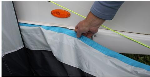
13. Finally - thread the draught skirt through the lower awning channel and secure at either side.
