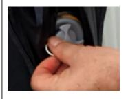
6. Replace the cap on the valve, before concealing it using the Velcro cover, in order to maintain a neater external aesthetic. Please repeat steps #3 to #6 for the remaining four tubes.
