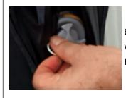
6. Replace the cap on the valve, before concealing it with the cover to maintain a tidier external aesthetic. Repeat steps #3 to #6 with the four remaining tubes.
