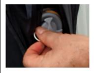
6. Replace the cap on the valve, before concealing it with the Velcro cover for a tidier external aesthetic. Please repeat steps #3 to #6 with the three remaining tubes.
