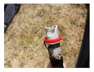
4. Insert the pump into the Dynamic Speed Valve and begin to carefully inflate, ensuring that none of the fabric is caught anywhere.
